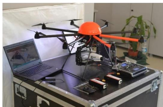
Figure 8. Octocopter with mounted hyperspectral camera
