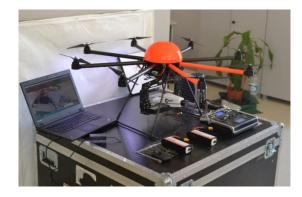
Figure 8. Octocopter with mounted hyperspectral camera
