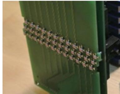
scanning area (240 mm wide), four detector panels are used, each of a width of 60 mm. In a whole, the device combines  $4 \times 36 = 144$  detectors which enable, with some margin, the analysis of the contains of the A4 envelope ( $210 \times 197$  mm).
