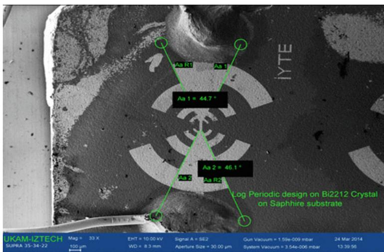
Fig. 12.3 SEM image of Log Periodic Antenna
