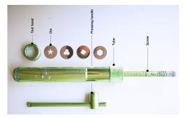
In the conventional use of the tool, first, the soft material is put in the tube and the die is placed into the tool head. When the handle is rotated, the disk pushes the clay down through the die to make the material dislodged. The output is a straight extrusion that is built layer by layer. It is cut to the defined length by a wire.
