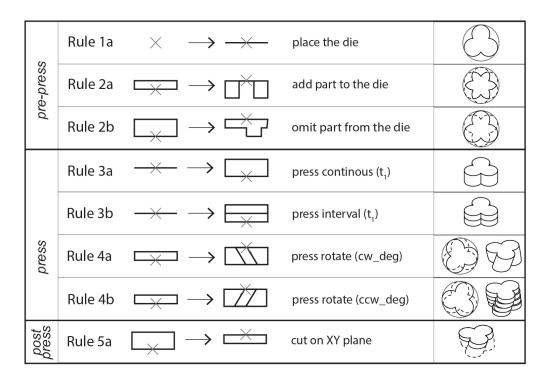
Figure 2 Extrusion-based making grammar (EbMG).
