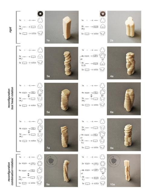
and 8a). The combination and rotation of dies also generate variation both in the section and the surface. As shown in Figure 5.9a, continuous press with 360 degrees of tool head rotation introduces variable grooves on the surface. The multi-step extrusion with equal press duration creates equally distributed partitioning on the form (10a).
