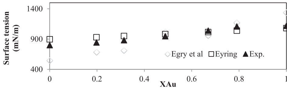
Figure 4. Surface tension of liquid Al–Au alloy as a function of the Au content for two models along with the experimental results at 1400 K. The experimental data are taken from Ref. [39].
