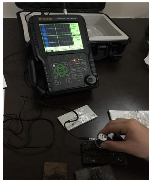
Figure 2: Ultrasonic examination of welded samples.
